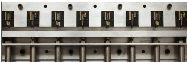
*Durability testing was conducted through an independent testing facility to determine the failure point of various mold counters. To view data, videos and more visit [www.procomps.com/CounterView](http://www.procomps.com/CounterView).*
