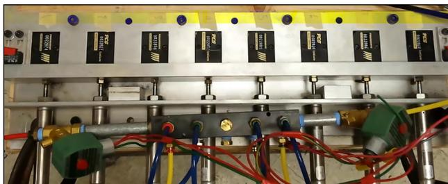
*Durability testing was conducted through an independent testing facility to determine the failure point of various mold counters. To view testing data, videos and more visit [www.procomps.com/CounterView](http://www.procomps.com/CounterView).*
